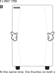
At the same time, the thumbs on both sides of the doors of buckle hole position, the index finger gently push the lid to the direction of the thumb. 左右手同時以大拇指按實機器門板的兩邊門扣孔位置,食指輕輕力把門蓋推向大拇指的方向。
