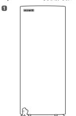
Press the button in the lower right corner to release the metal sheet hole's lock. 按一下右下角金屬片的按鈕,即可鬆開鎖扣。
