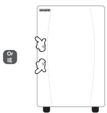
At the same time, the thumbs on one side of the doors of buckle hole position, the index finger gently push the lid to the direction of the thumb. 左右手同時以大拇指按實機器門板的一邊門扣位,食指輕輕力把門蓋推向大拇指的方向。
