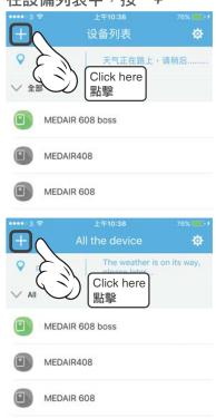
2 Before the wifi connection, press the UV and plasma ion together in standby mode, until you hear a "tick" sound then scan QR code to connect your air purifier.
