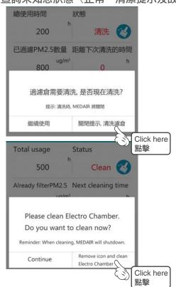
● Fault prompt / function page & press inquire to check status (normal, cleaning & fault) 故障提示 / 進入功能頁,然後按查詢來知悉狀態(正常、清潔提示及故障提示)
